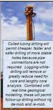
Coiled tubing drilling will permit cheaper, faster and safer drilling of more stable holes because pipe connections are not required. Logging-while-drilling will remove or greatly reduce need for core and lengthy core analysis. Combined with real-time geological modelling, these will permit follow-up drilling without rig de-mob and re-mob.
