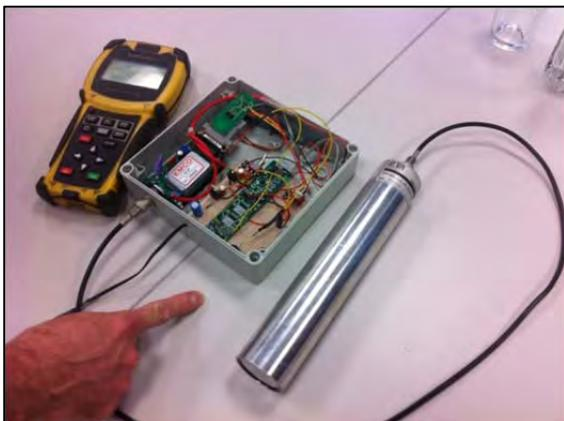
Initial circuitry and sensor for world's first LWD system for minex: to be housed in autonomous shuttle and deployed in rods (Project 2.2).
