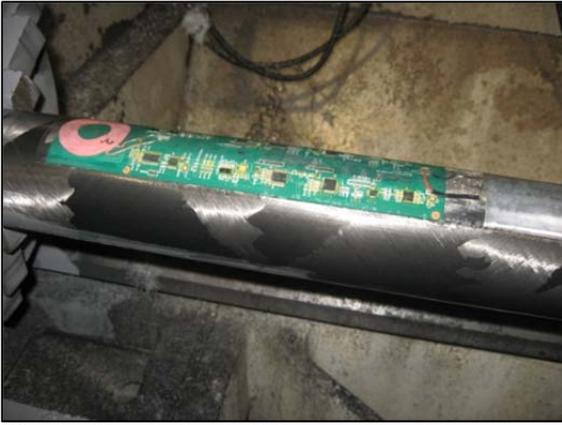
*NO carbon fibre rod with embedded core orientation electronics.*
